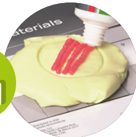
Fig. 49–51: Correctly dosed strands (left). In comparison, unevenly and too thin (middle) respectively too thick dispensed strands (right).
