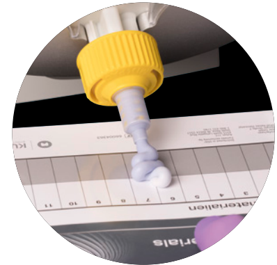
Fig. 38: Discarding of the initial 2–3 cm to adjust the filling levels of the two material components.
