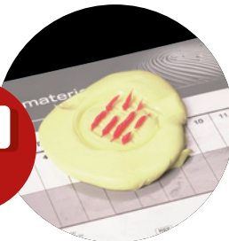
Fig. 49–51: Correctly dosed strands (left). In comparison, unevenly and too thin (middle) respectively too thick dispensed strands (right).
