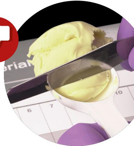
Fig. 44: Removal of the excess material in one go should be avoided as the material can be pushed out from the spoon resulting in underdosing.
