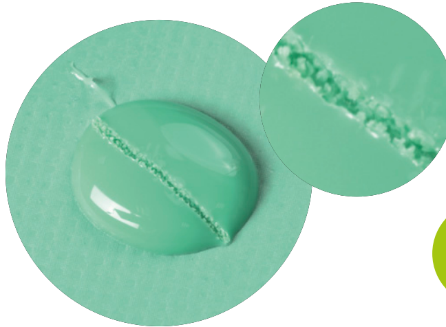
Fig. 22: Absence of an unpolymerized layer (smear layer) shows compatibility of the used materials.
